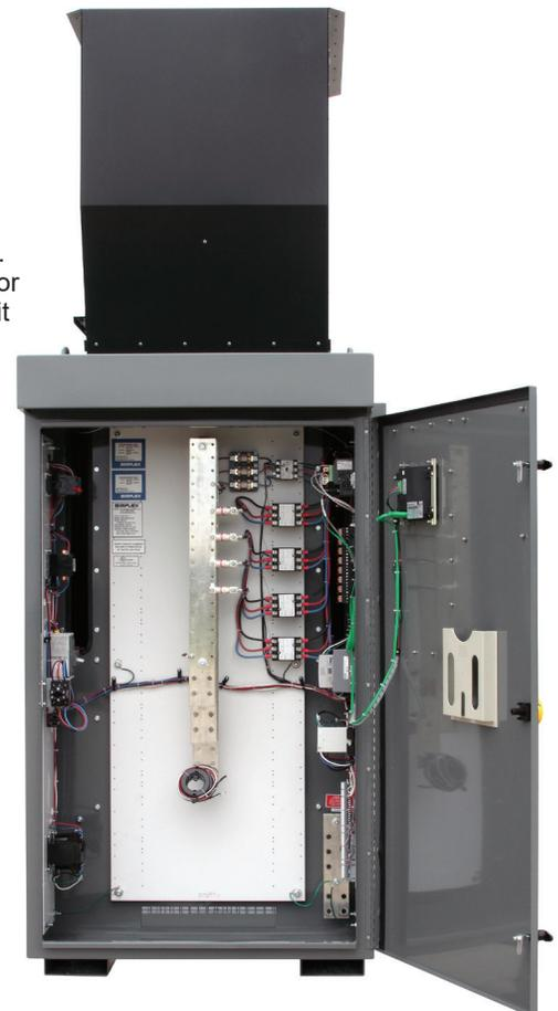
The load bank enclosure is of double wall construction for cool exterior and thermal isolation of the load elements. Cooling airflow through the enclosure is vertical with cold air intake at the bottom and hot air exhaust out the top. Intake and exhaust openings are screened. Enclosure is powder-coated dark gray. Hood powder-coated high temperature black.
