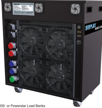
Infinity-200 or Powerstar Load Banks can be networked together via RS-232 cables connected from the "out" connector on the first unit to the "in" connector on the next, and then "out-to-in" in succession until the desired number of units are connected. All control and metering is provided from a single hand-held controller. All instrumentation values for the total network are summed and displayed on the master controller.
